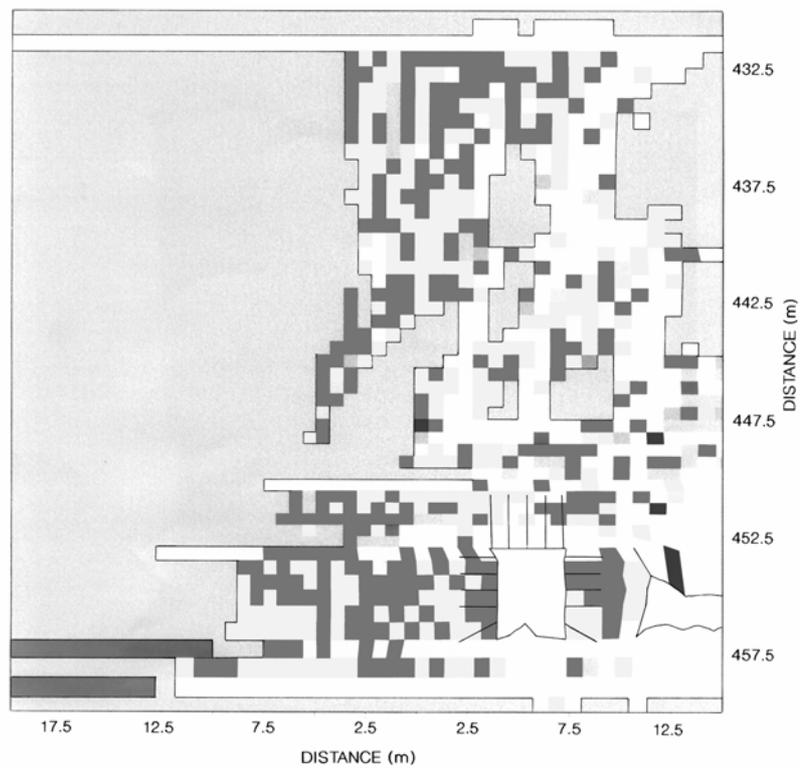
**Fig. 6(b) –Rock Failure about a 4m pillar – high strength bolts,
