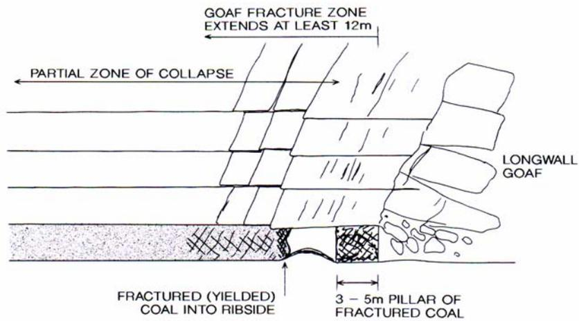
**PROBLEM:** Potential collapse of broken strata above roadway if the small pillar loses strength
