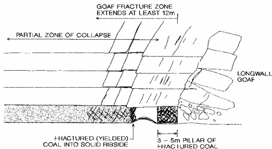
**GLOBAL STABILITY ISSUE:** Potential collapse of broken strata above roadway if small pillar loses strength
