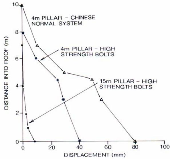
**Fig. 8(a) – Roof behaviour for various options at Dongpang Coal Mine.**
