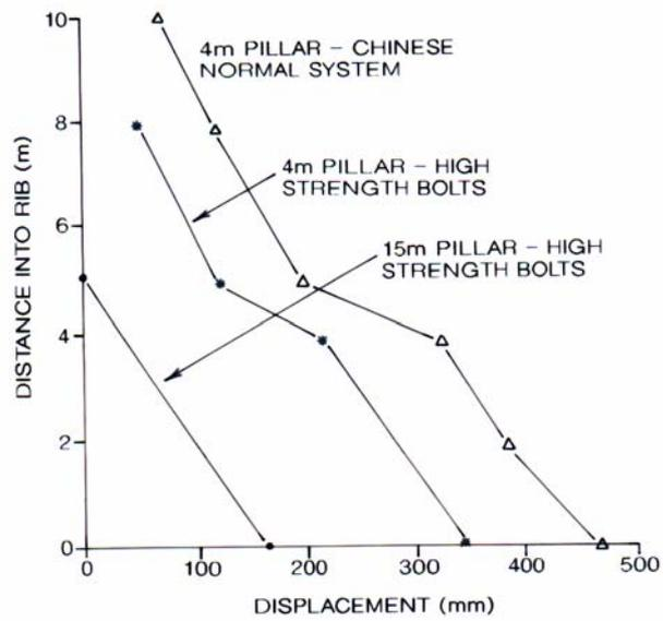
**Fig. 8(b) – Rib behaviour for various options at Dongpang Coal Mine.**
