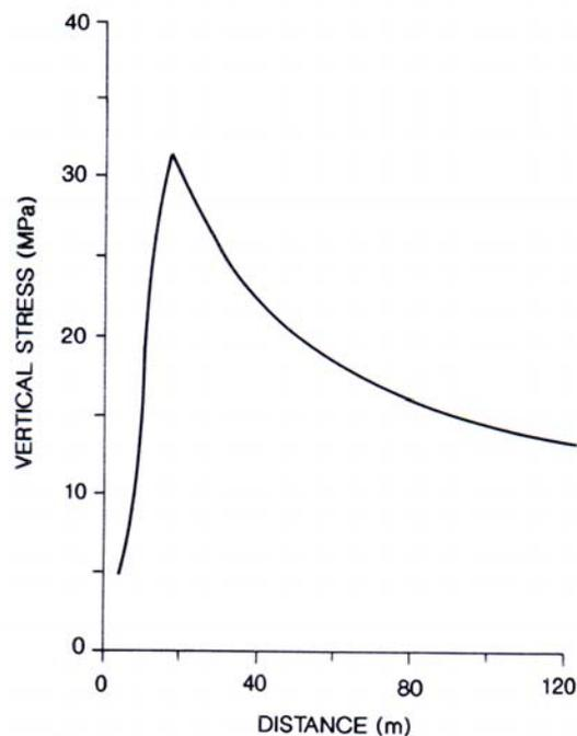
**Fig. 5(b) – Vertical stress abutment from Longwall 2705 at Dongpang Coal Mine.**
