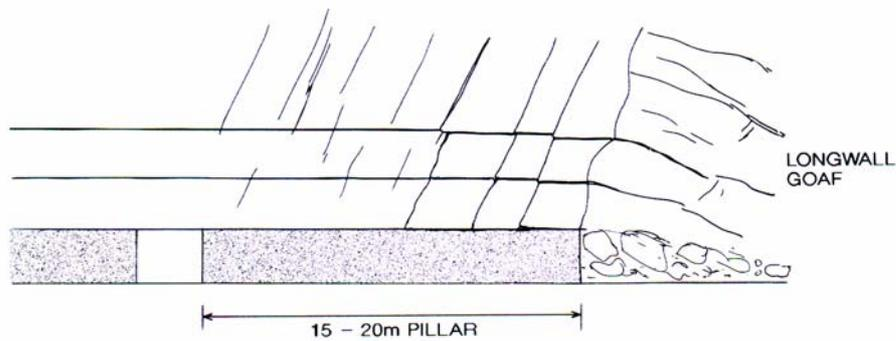
**SOLUTION:** Improved safety of the roadway with the use of a larger pillar to isolate the roadway from goaf collapse
