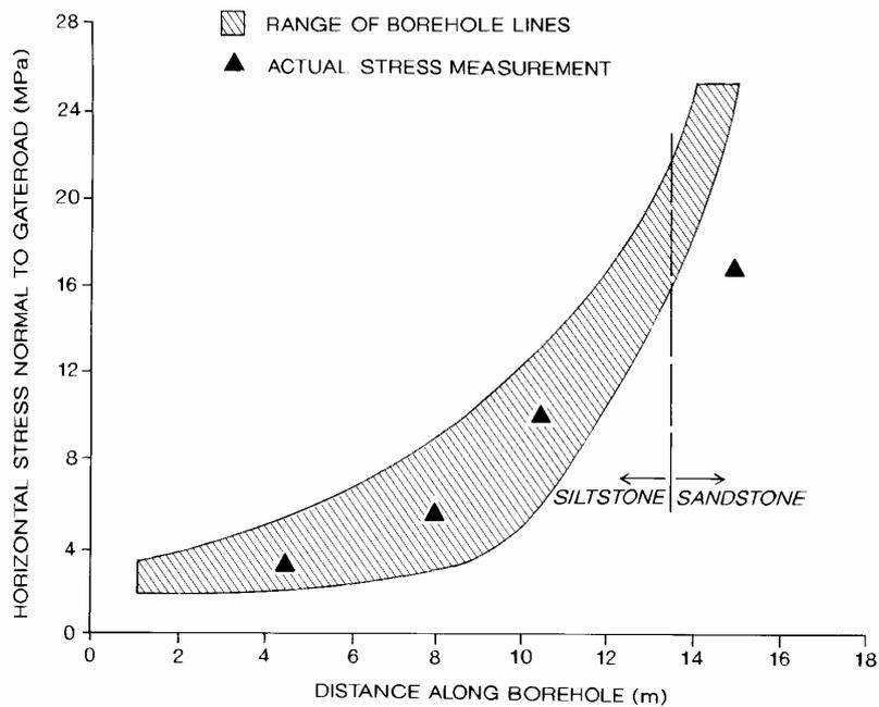
b) Comparison of modelled and measured horizontal stress.
