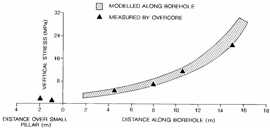
a) Comparison of modelled and measured vertical stress.
