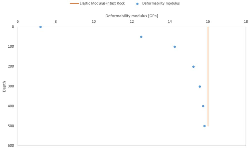
Figure 7: Variation of deformability modulus with depth
