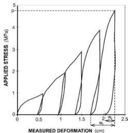
Figure 1: Typical loading response of jointed rock
