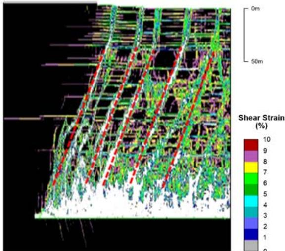
**Figure 7 Generic numerical model of longwall caving showing cyclic overburden caving fractures.**
