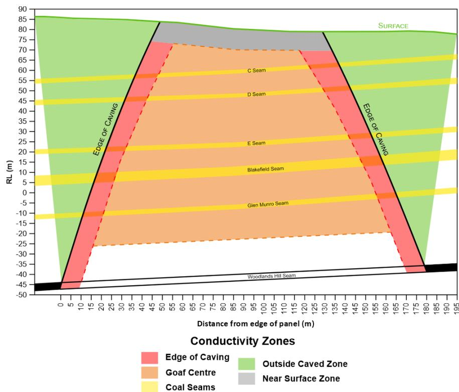
**Figure 6 Hydraulic conductivity zones above Longwall 10.**
