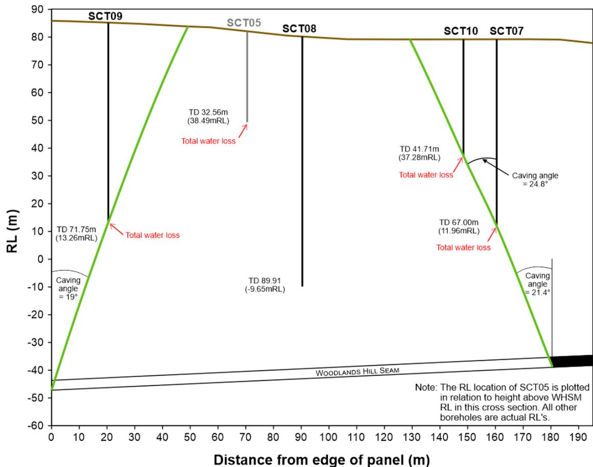
Figure 3 Inferred edge of caved zone from drilling results.
