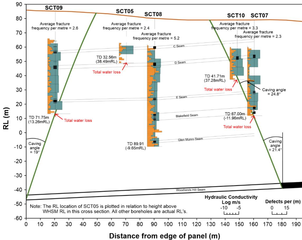
**Figure 5 Drilling and hydraulic conductivity results in relation to caved zone.**
