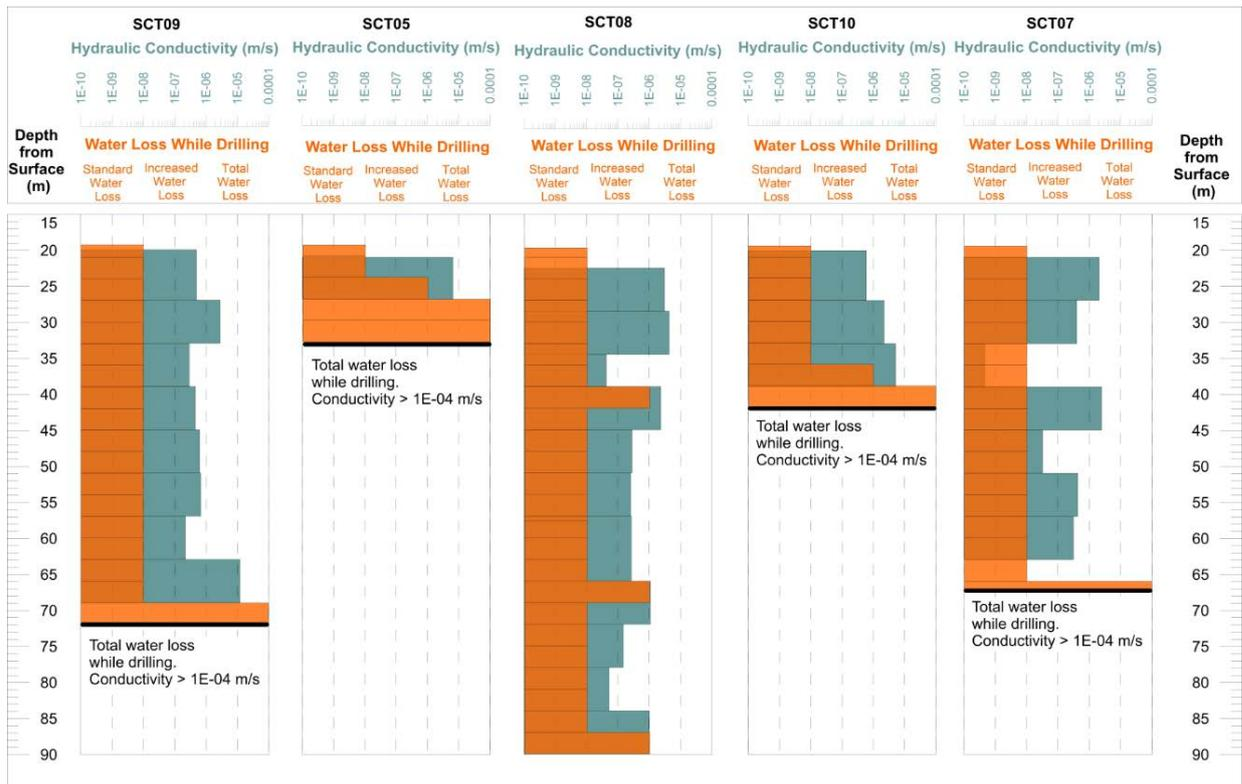
**Figure 4 Hydraulic conductivity results and water loss zones over Longwall 10.**
