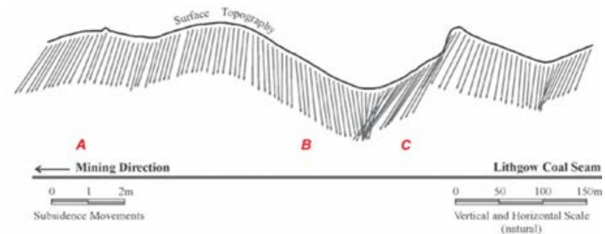
a) Vertical section showing longitudinal displacement vectors.
