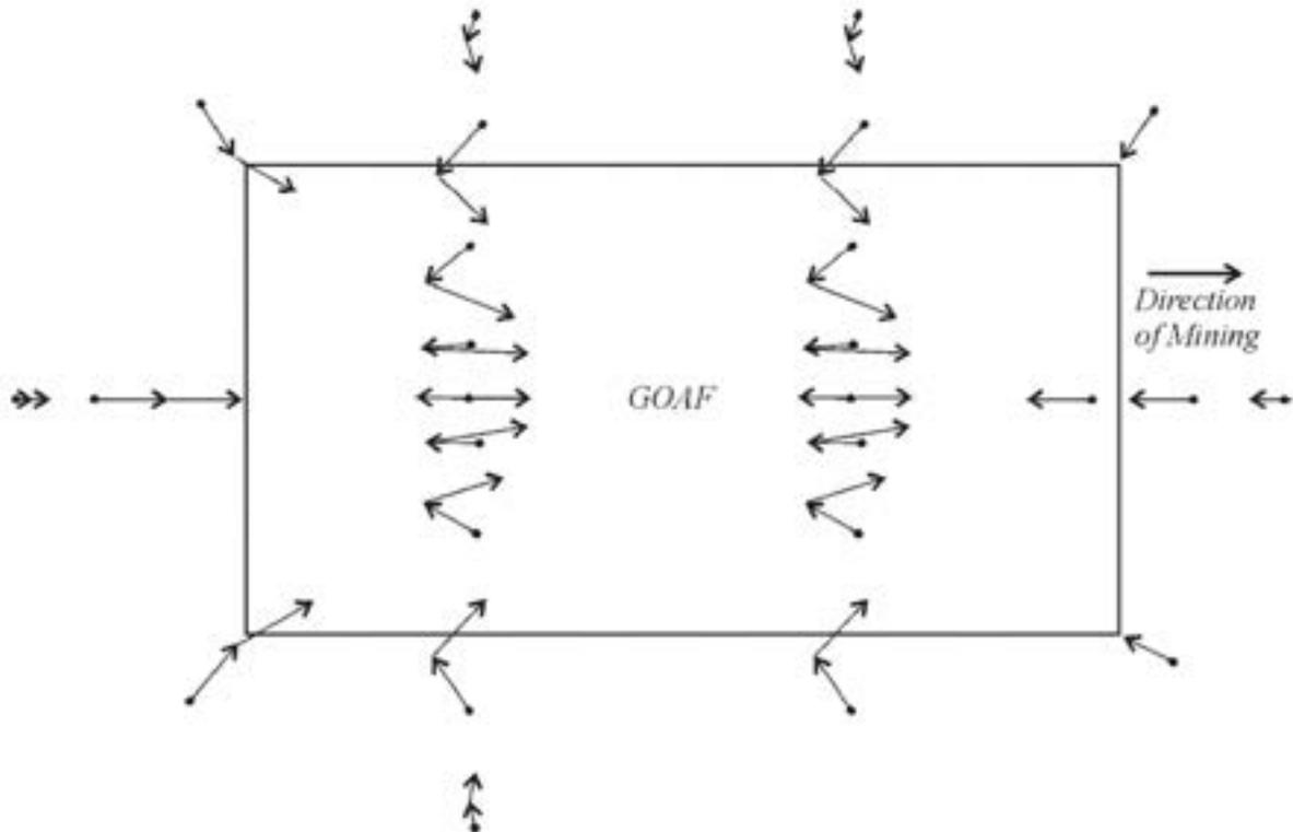
**Figure 7 Systematic horizontal movements around an extracted longwall panel in flat terrain (after Mills 2001).**
