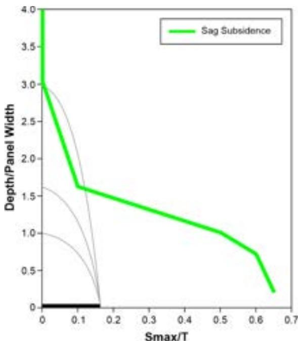
**Figure 3 Subsidence experience shown in Figure 2 replotted with axes reversed and panel width to depth ratio inverted (after Mills 2012).**
