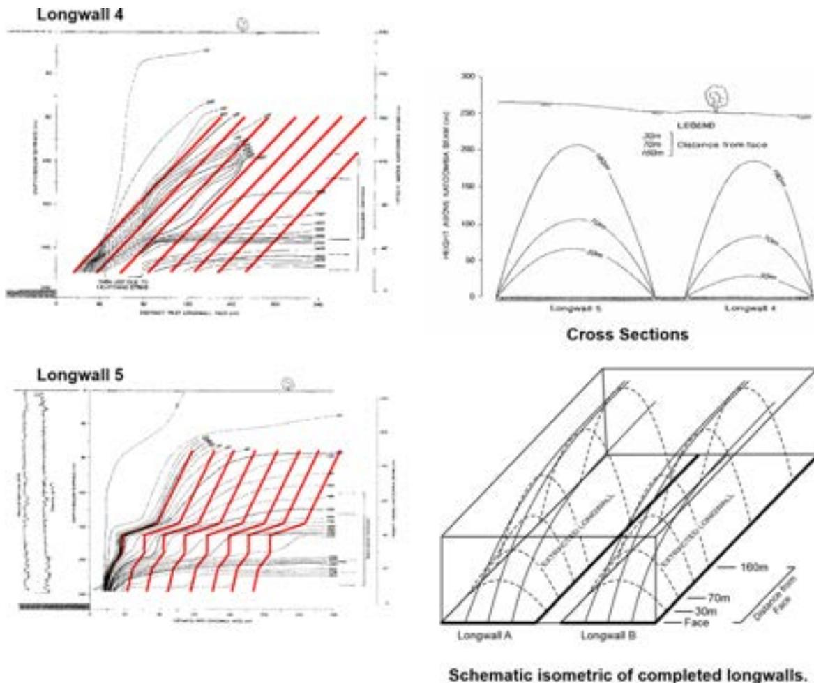
**Figure 11 Fracture pattern (in red) within the zone of large downward movement indicated by extensometer monitoring above a retreating longwall face (after Mills and O'Grady 1998).**
