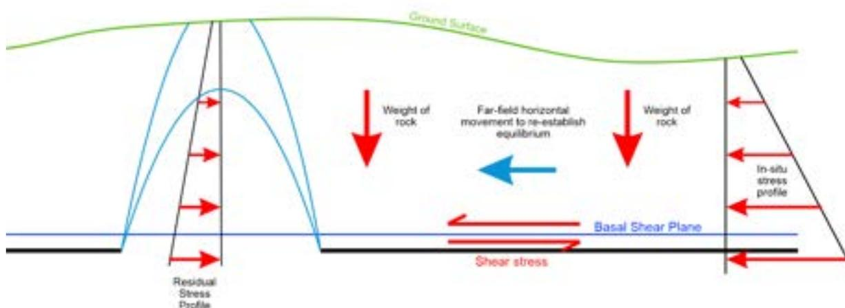
**Figure 8 Mechanics of process that causes far-field horizontal movements associated with stress relief.**
