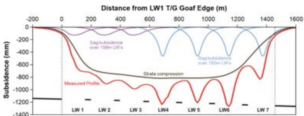
**Figure 6 Sag and strata compression subsidence components of the measured subsidence profile.**
