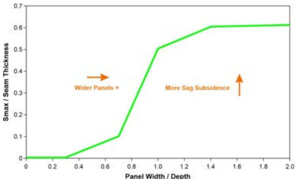
**Figure 2 Sag subsidence plotted conventionally as the ratio of maximum subsidence divided by seam thickness plotted against panel width to depth ratio.**
