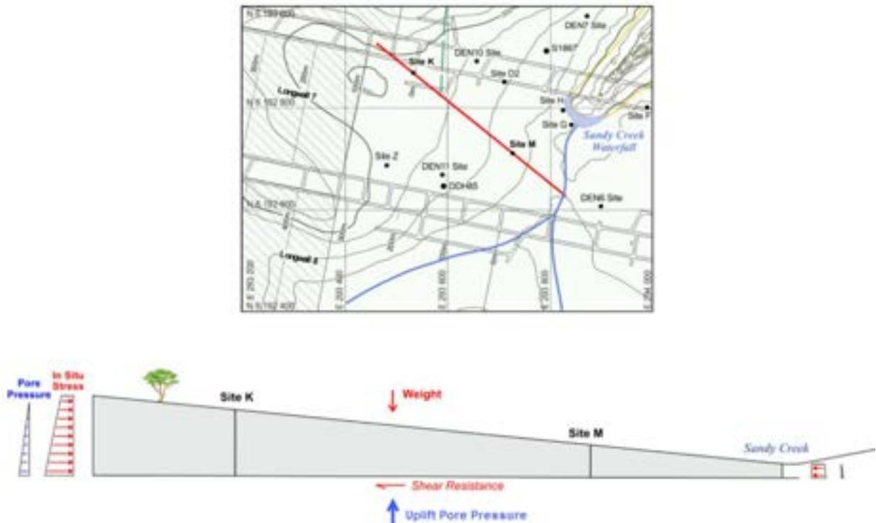
**Figure 10 Free body diagram of slope leading down to Sandy Creek that shows friction angle on the basal plane is in the range  $9^{\circ}$ - $14^{\circ}$  (after Walsh et al. 2014).**
