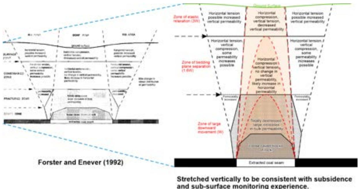
**Figure 12** Zone of permeability change indicated by Forster and Enever (1992) are consistent with subsidence and sub-surface observations when stretched vertically as shown.
