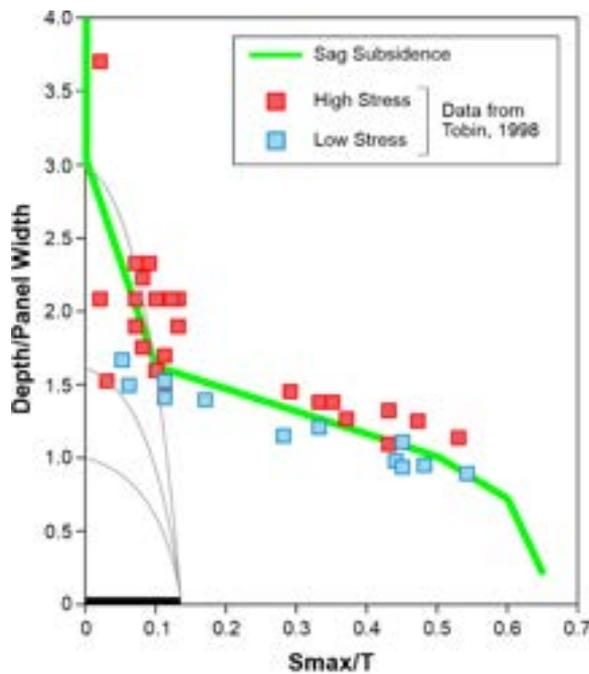
**Figure 4 Subsidence from longwall panels in the Newcastle area oriented across and parallel to the major horizontal stress (after Mills 2012).**
