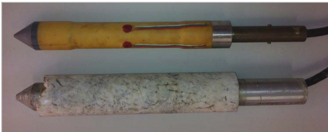
Figure 1: Photograph of original ANZSI strain cell design and overcore in gneiss.
