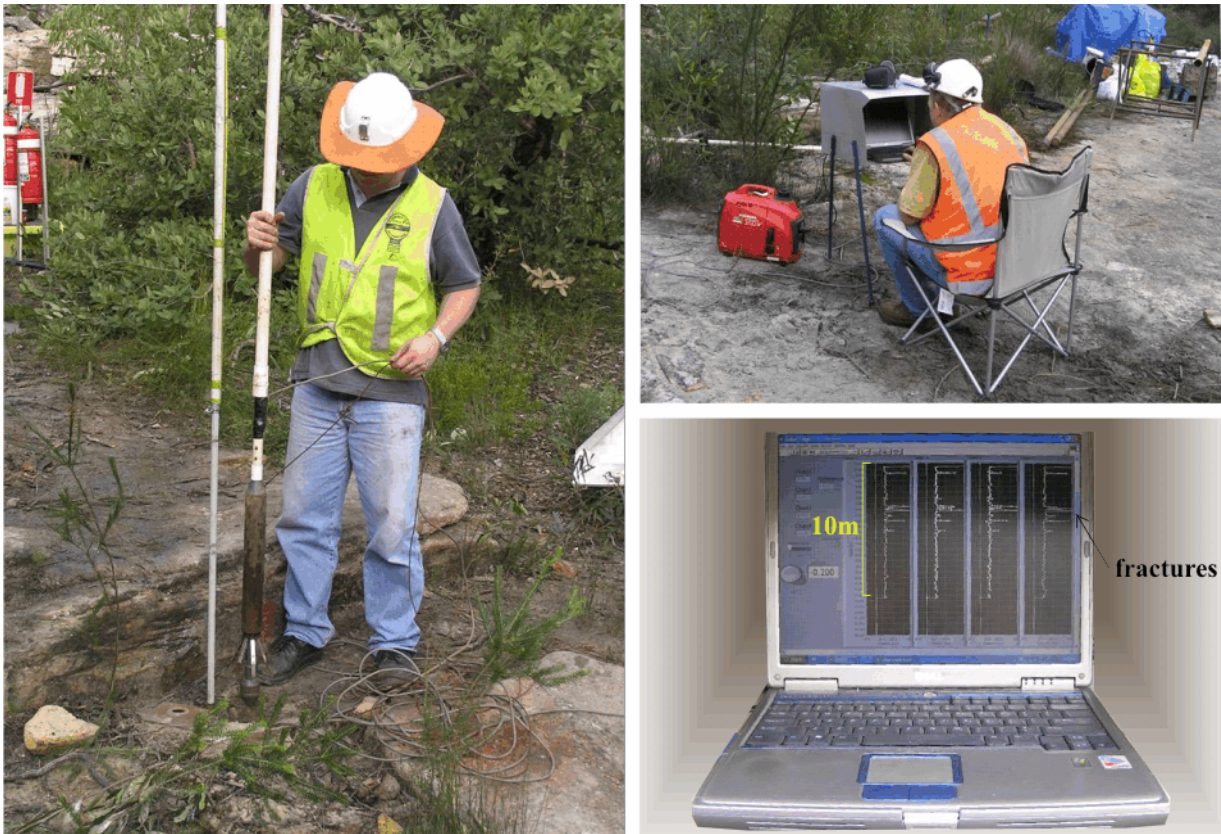
Fig 2: Caliper logging system for fracture measurement.
