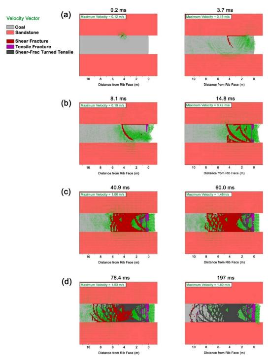
Figure 3: Development of coal burst phenomena over time.
