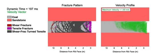
Figure 6: Final fracture pattern and velocity profile produced by DRFM<sup>2D</sup>
