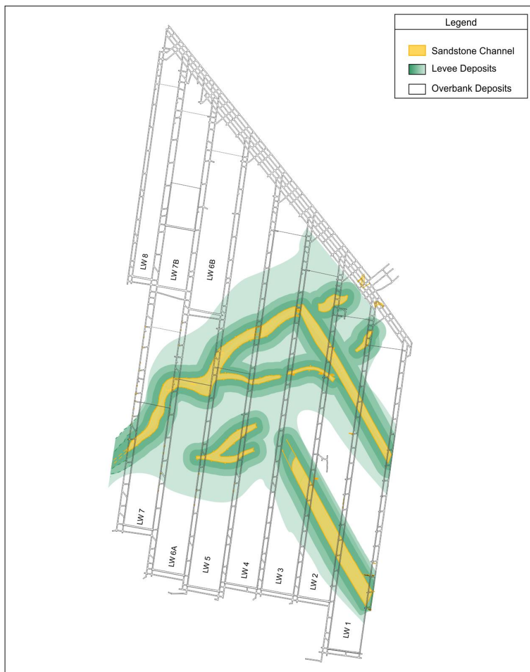
Figure 5 - Distribution of mapped channel exposures and distribution of levee deposits in Ashton underground roadway development headings
