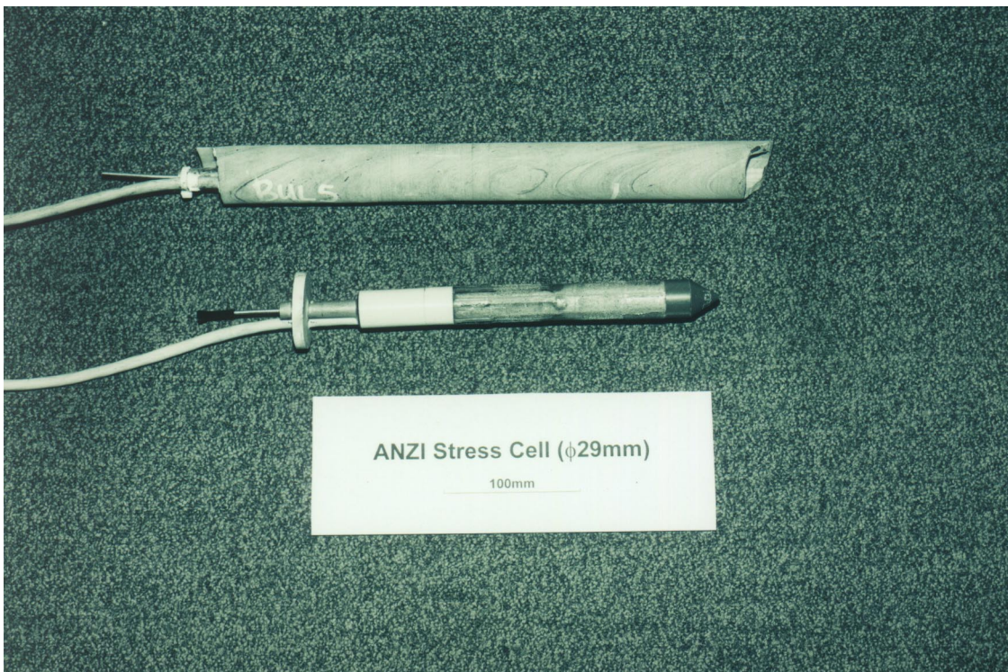
Figure 3. 29 mm diameter version of the ANZI with a 42 mm diameter overcore in sandstone
