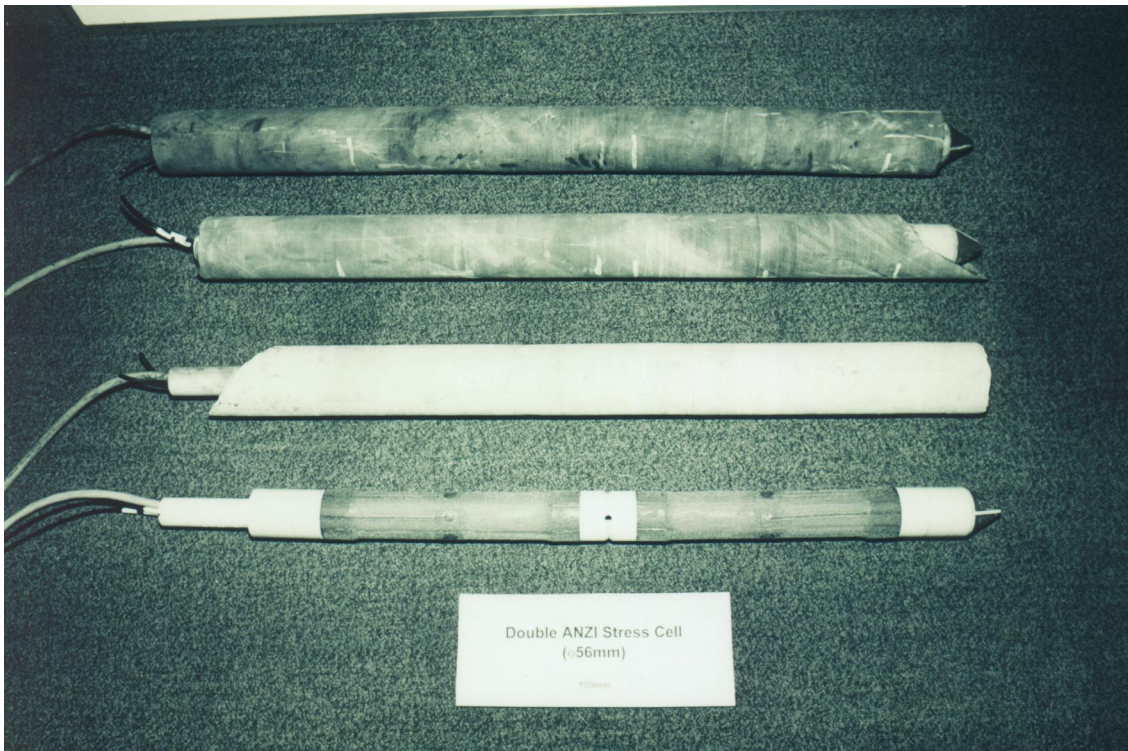
Figure 2. Double ANZI configuration showing instrument and overcores in various coal measure strata
