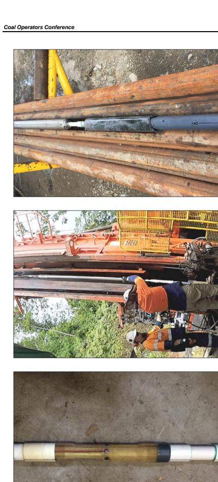
b) Deployment assembly, downhole logger and ANZI strain cell immediately prior to installation.
